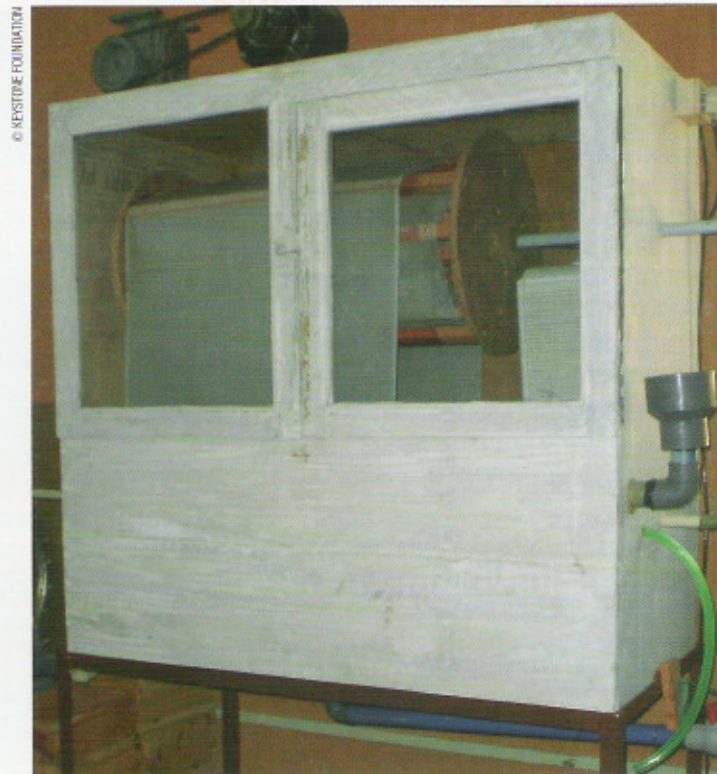
In the chamber of the honey dryer, honey constantly moves on a thin nylon film and water content is reduced without raising the temperature of the honey
